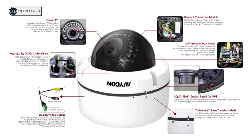
Vandal Proof Dome The camera housing is made with industrial strength steel-alloy metal with high quality poly-carbon dome cover protecting from most severe vandalism.
